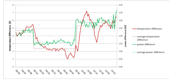
Figure 8: Exemplary temporal course of temperature and power difference comparing normal cell strings to those with thermal anomalies
